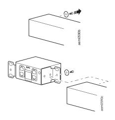
Secure the coupled Rack Access Pod and Sensor Pod to the rack using cage nuts and screws (not provided).
