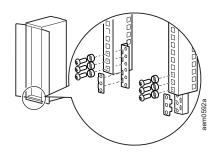
Use the provided M6 screws and washers to secure the coupled Rack access pod and sensor pod to the rail extender.
