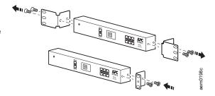
4. Remove one peg and screw from the Sensor Pod 150. Then use the peg and screw to secure the Rack Access Pod to the Sensor Pod 150.
